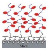
Robust polymer brushes are grown from a planar mica surface (see figure) using atom-transfer radical polymerization. The brushes are characterized by X-ray photoelectron spectroscopy, X-ray reflectometry, atomic force microscopy, optical interferometry, and surface forces.
